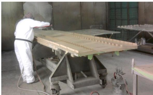
*The Chromium-Free Wash Primer Replacement Team applies hexavalent chromium-free alternatives to DOD-P-15328 wash primer to metal coupons in preparation for performance testing.*
